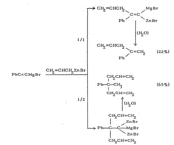
With vinylic organometallic reagents an exothermal addition takes place at  $35^{\circ}$ , e.g. [46]:
